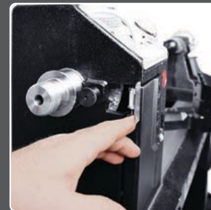
Spindle indexing in 24 points
