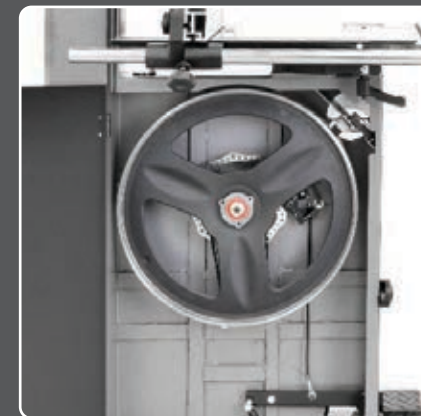
Foot pedal brake quickly stops the belt
