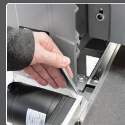
Index lever will properly adjust the conveyor to give a seamless finish
